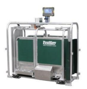
The Prattley Electric AutoDrafter is operated by electric motors powered by a 12volt battery, and will operate on a fully charged battery for a full day. The design eliminates the need to have left or right handed crates. The rear gates have vertical rollers which allow the gates to roll around the sheep as they close or allow the following sheep to pull back without getting caught.
